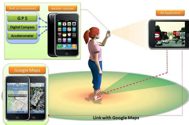
Figure 4 Architecture of Acrossair's augmented reality applications.
